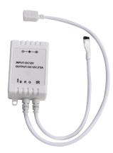
Create custom lighting effects with this 44-key IR remote control and LED control unit, that's specifically designed to work with 12-24 VDC RGB LED light ThinGlow strips. Adjust brightness, color, fade in/out, and flash rate. Supports up to five meters of RGB LED light strips. Other tri-color, common anode LEDs may be used if configured to work with 12-24 VDC supply voltage by the use of voltage dropping resistors. IR remote control uses a CR2025 battery (included).
